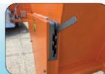
Spring stone release and extract chute adjustment
