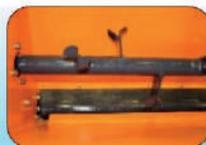
Lump actuator and spreading roller
