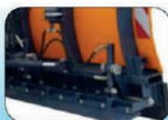
Rubber&Hardox cutting edges
